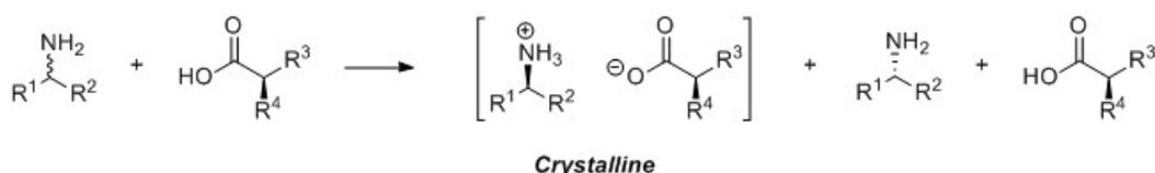
**Scheme 1: Chiral amines are obtained in industry by co-crystallisation with chiral agent**
